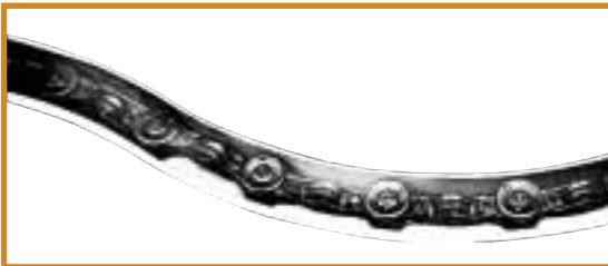
Looking through side of track. Track cut-away of chain passing through reverse vertical curve.
