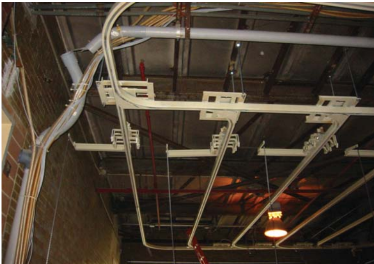
Richards-Wilcox Conveyor, Frog Switches divert to multiple lanes for laundry accumulating
