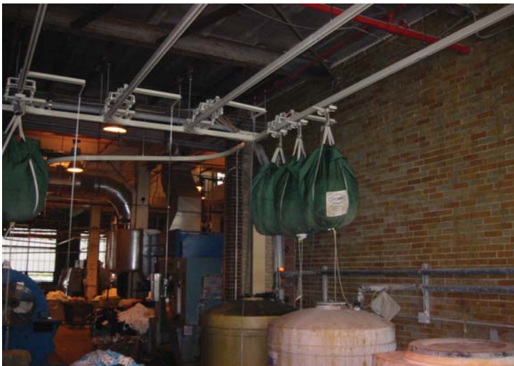
Richards-Wilcox Conveyor, Multiple laundry lanes accumulating bags.
